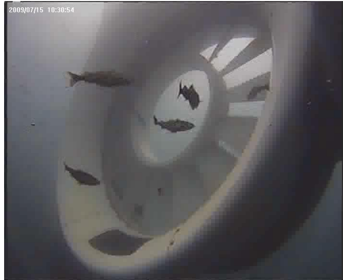
Figure 3 – Unlighted video observation of OpenHydro turbine at EMEC. In this image, fish are aggregating downstream of the turbine. Current velocity is below cut-in speed for the turbine.
