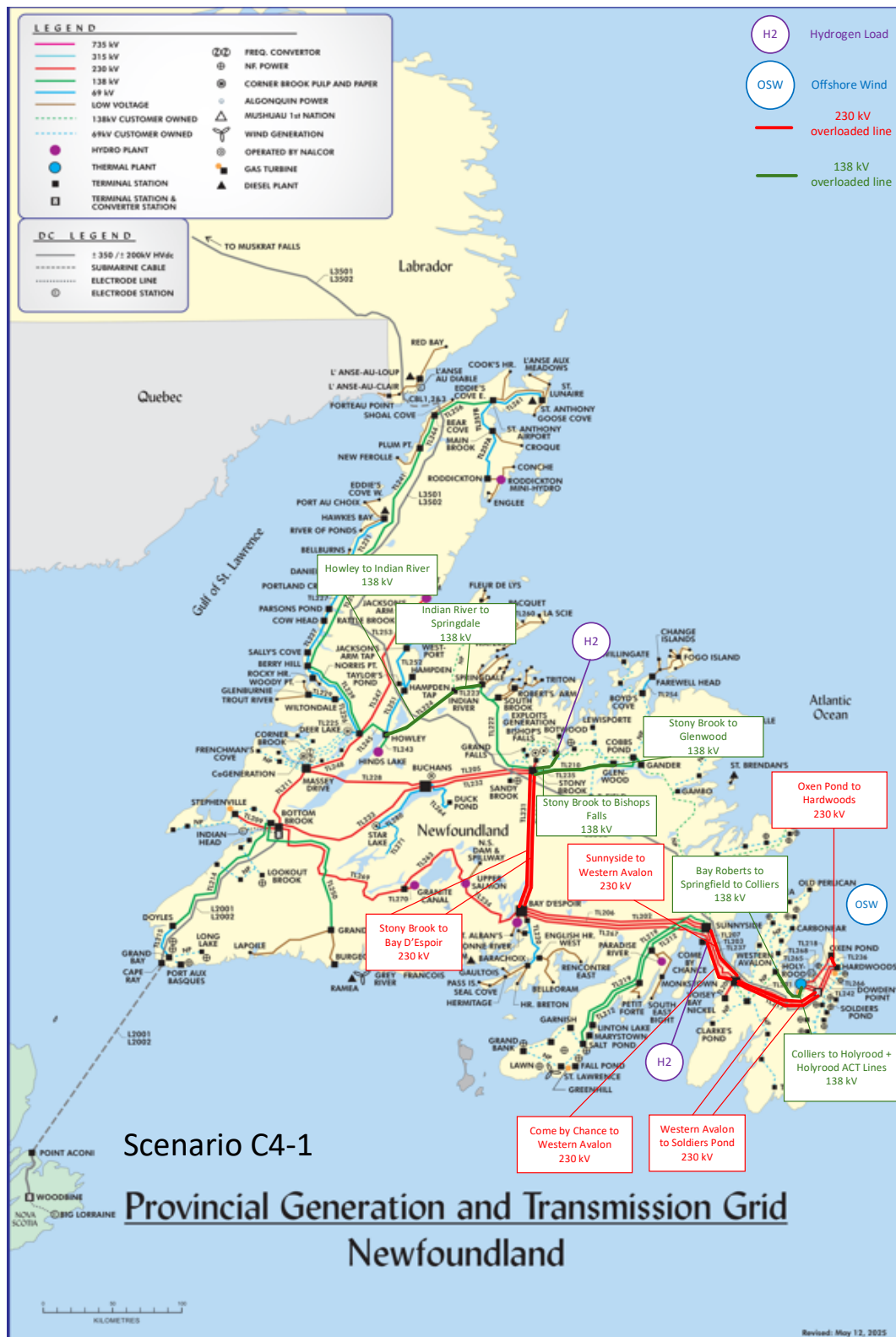
Figure 6.R Scenario C4-1: Key System Overloads in Newfoundland and Labrador
