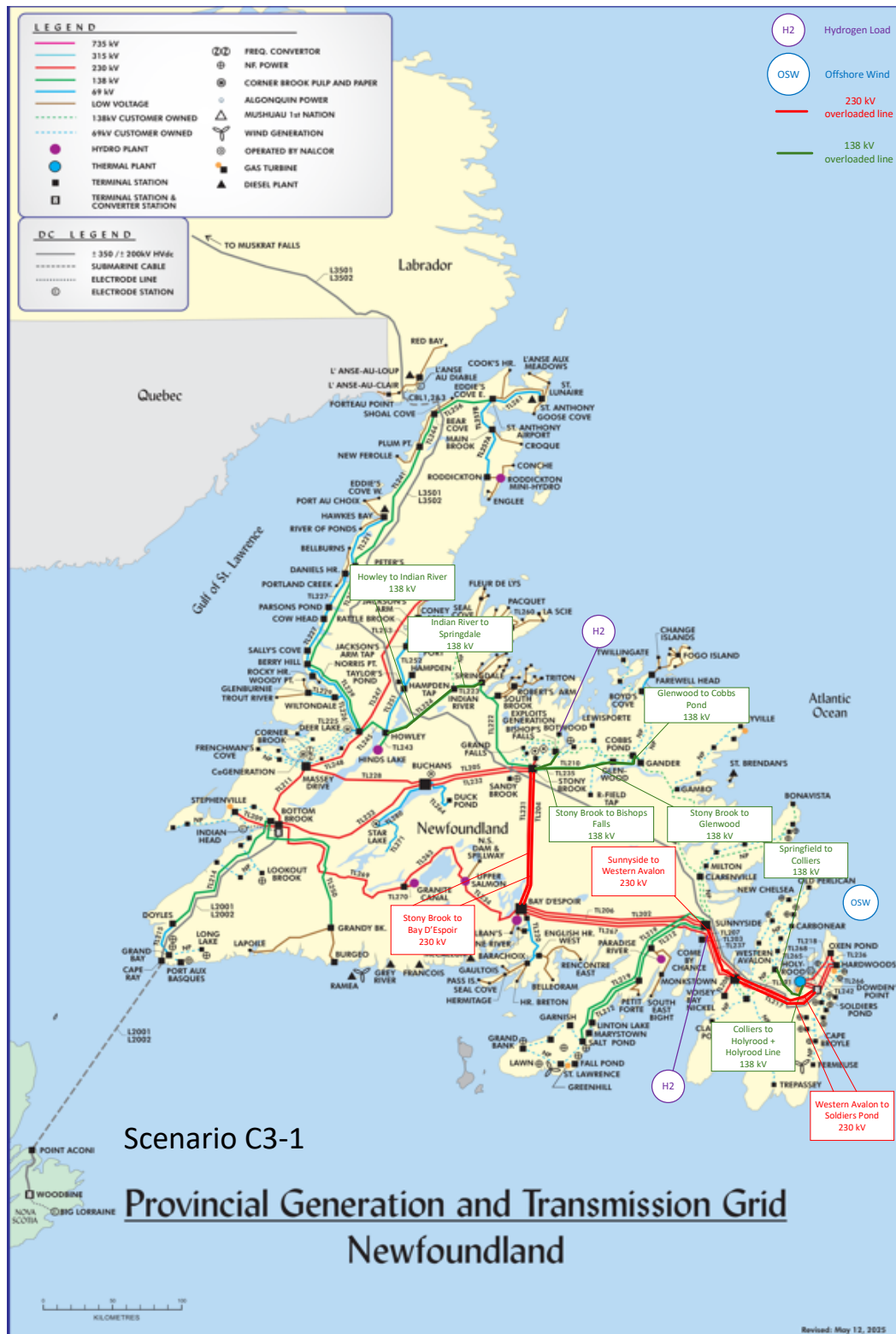
Figure 6.O Scenario C3-1: Key System Overloads in Newfoundland and Labrador
