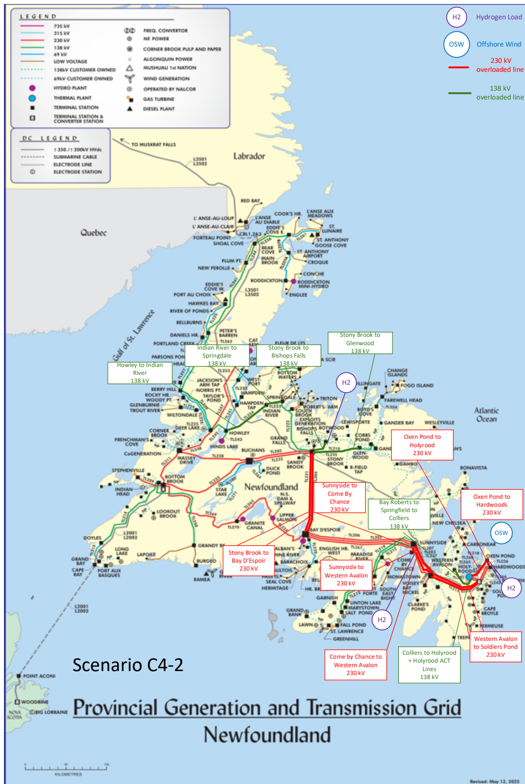
Figure 6.U. Scenario C4-2: Key System Overloads in Newfoundland and Labrador
