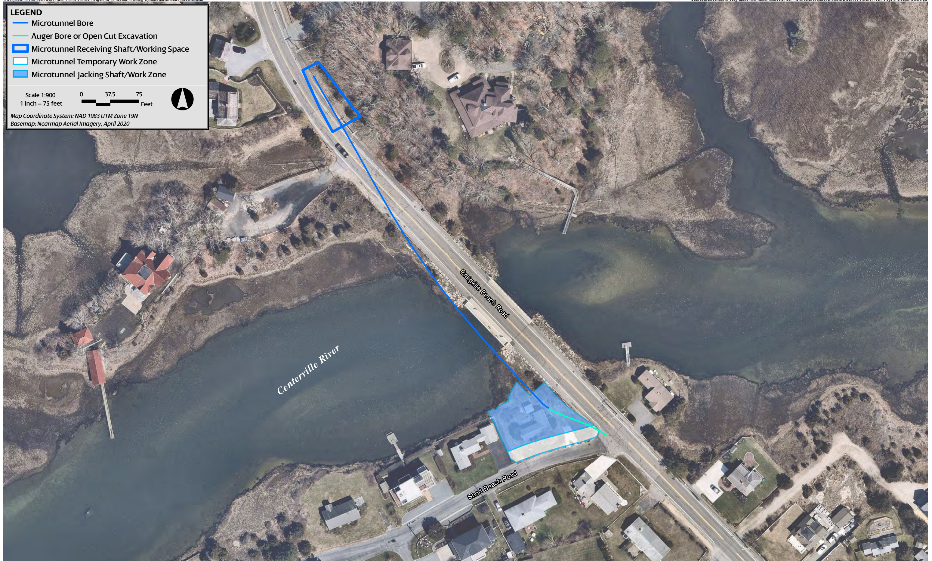
Figure 3.3-5a Centerville River Crossing Options (Microtunnel)
