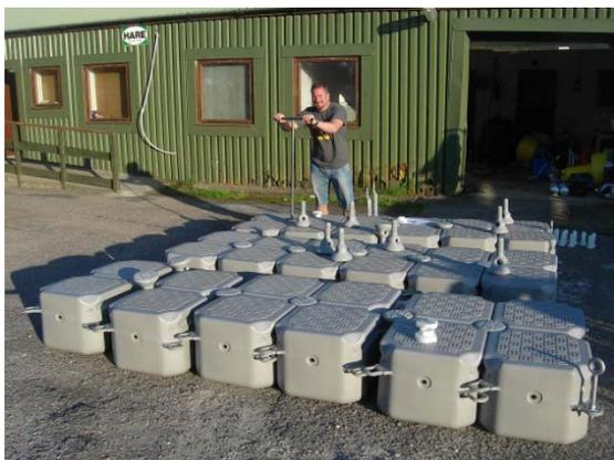
**Figure 5: Assembly of platform.**
