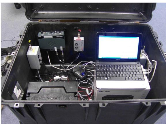
Figure 8: Pelicase containing equipment for sound recording.
