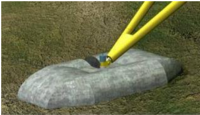
Plate 4.1 Gravity base 'foot'. (Image source – Tidal Stream limited)
