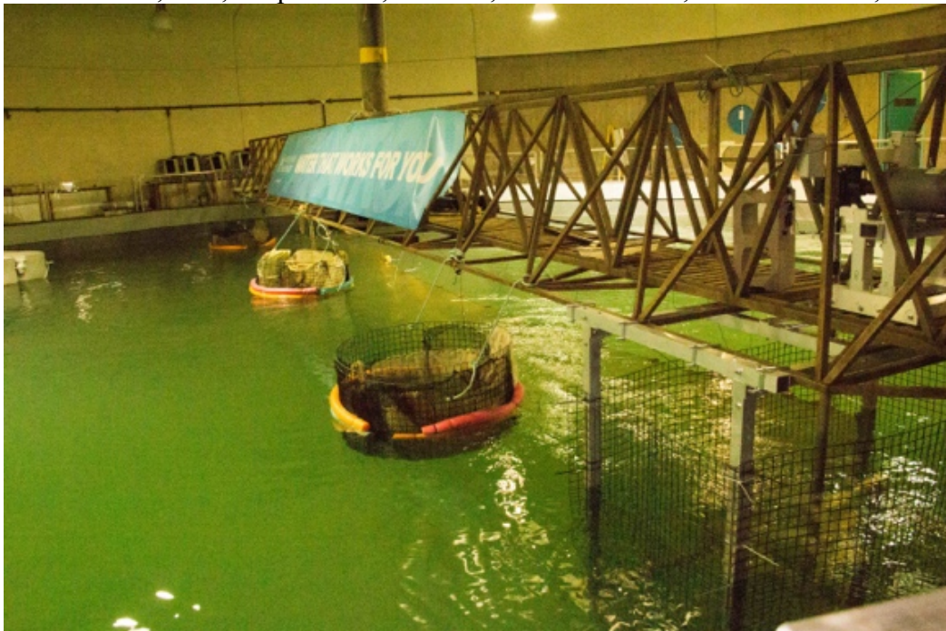
Figure 1 Tidal turbine and fish study experimental setup
