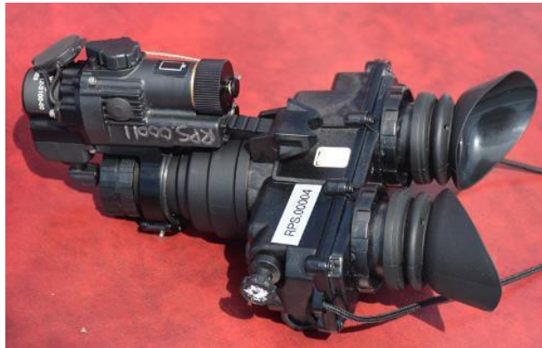
Figure 1: Night vision goggles with thermal clip.
