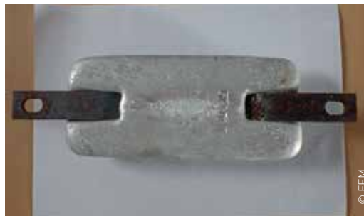
Figure 1. Example of galvanic anode cathodic protection
