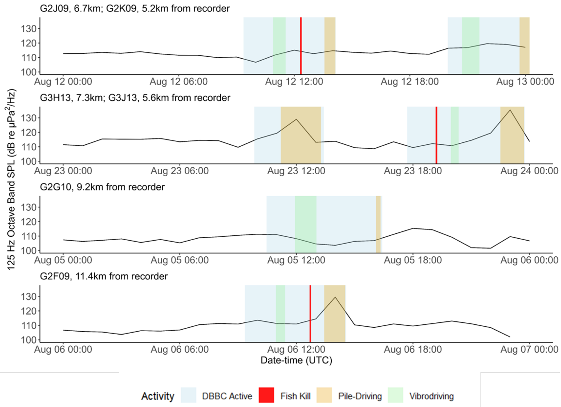
Figure 7. Daily time series of observed 125 Hz Octave Band SPLs visualized with shading indicating the associated construction activity that was occurring during specific monopiles installations (Note that the first two time series contain multiple piles). Note that the DBBC was also on while impact pile driving and vibratory pile driving were occurring.
