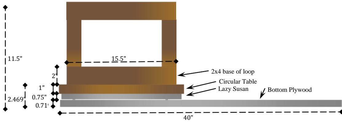
Figure 1. Diagram showing coil housing and rotating platform.
