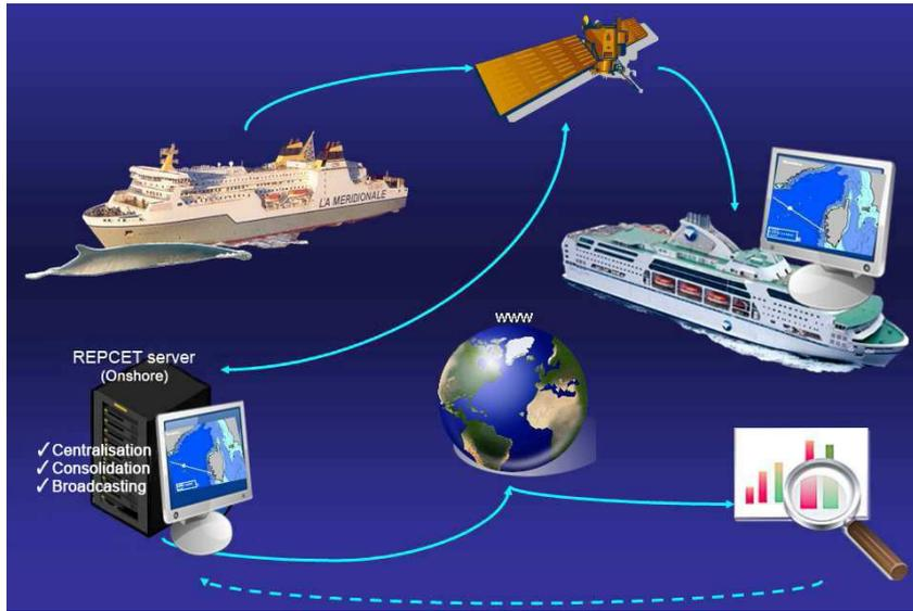
The REPCET tool is a software system dedicated to commercial navigation. Its aim, first and foremost, is to limit the risks of collision between large cetaceans and commercial vessels.
