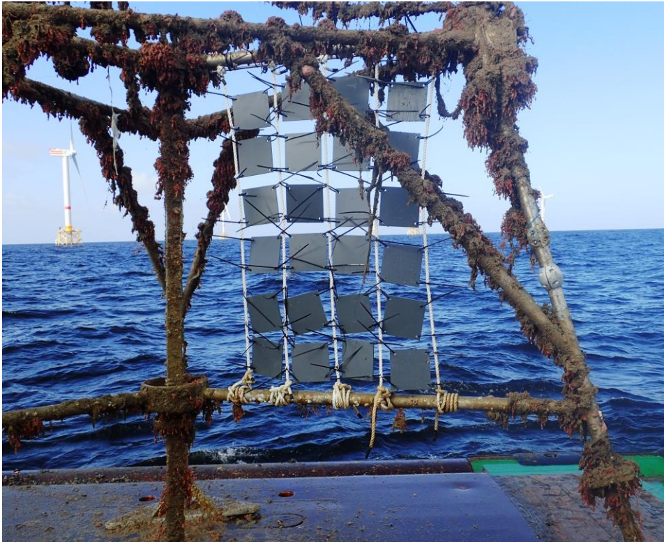
Figure 4.1: Image of the set-up of the PVC panels on the tripod before they were deployed at sea in April 2017.
