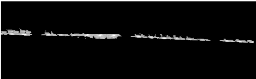
Fig. 3. A VPS image formed by combining the sequence of frames in Fig. 1 into a single image that retains the peak value of each pixel location. The background is removed by thresholding the pixel values.
