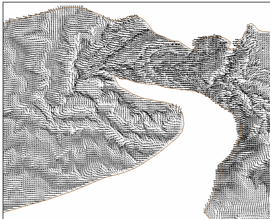
(b) Plot of current vectors in Minas Channel, Minas Passage and the entrance to Minas Basin
