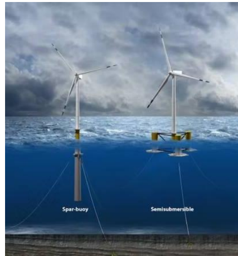
Figure 2: Visualization of floating structures used to founder FOW turbines. The spar-buoy on the left is an example of the foundations used at Hywind Scotland. The semi-submersible on the right is an example of the foundations used at Kincardine wind farm (after [14]).
