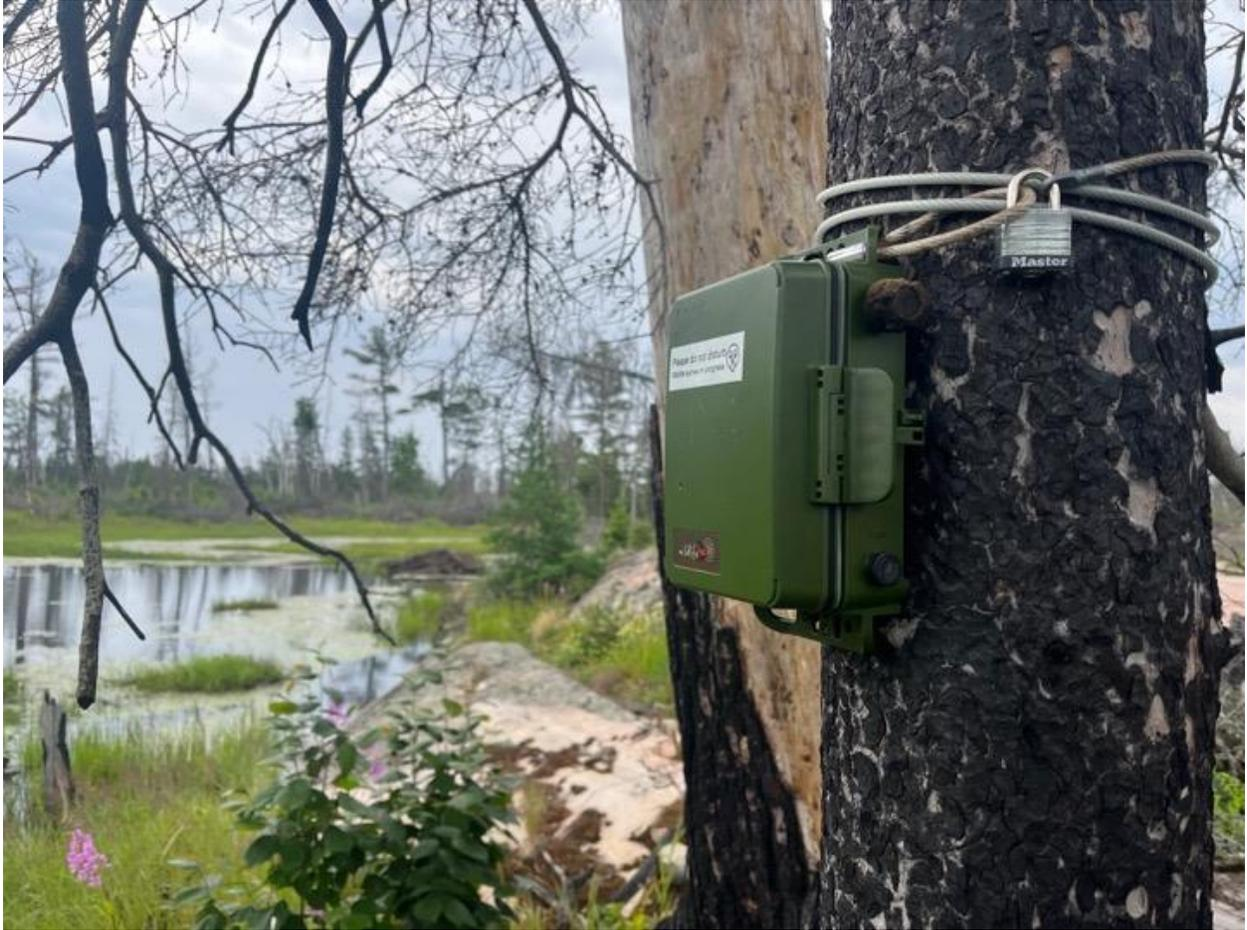
Appendix B: ARU (autonomous recording unit) attached to a charred tree adjacent to a wetland containing calling anurans, at a Burn treatment site.
