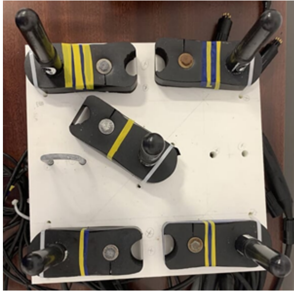
Fig. 2.6.2: A 5-element horizontal array
