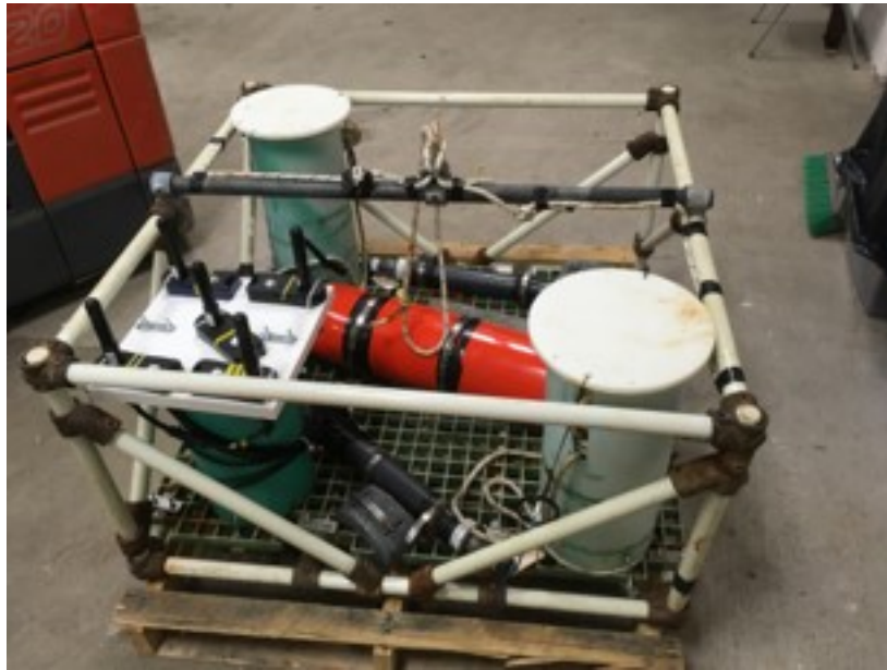
Fig. 2.6.3: Installation of the hydrophone array and acoustic releases in a frame.
