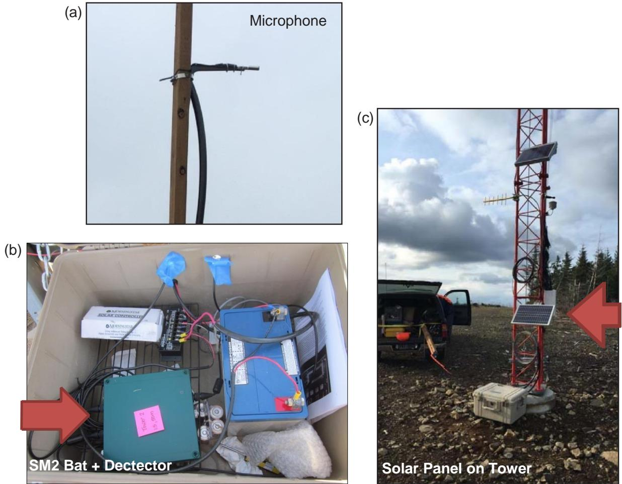
Figure 3. Photographs of bat acoustic monitoring equipment depicting a) microphones used at ground and meteorological tower locations, b) SM2 Bat + detector and solar battery housed in a waterproof Pelican case, and c) solar panel secured to tower.
