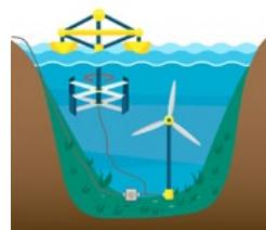
**River current energy** harnesses the steady flow of rivers without using dams.
