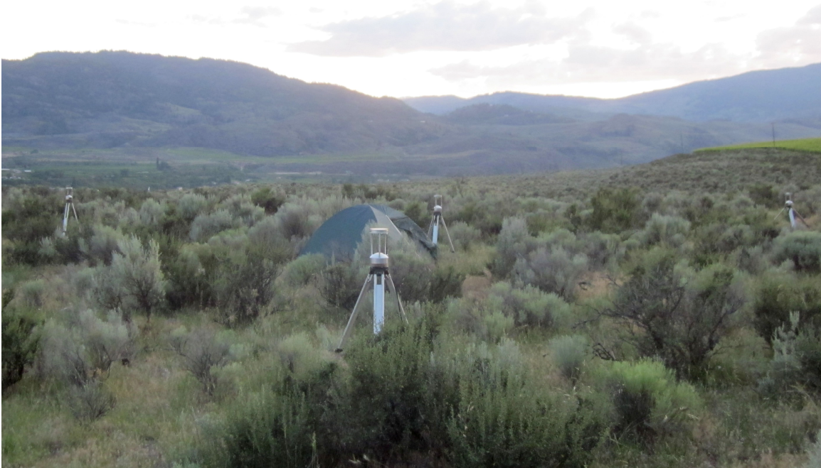
Figure 2.4. Overview of the bat acoustic array setup in one of my natural plots. The image shows the unique design of the EchoTrack omni-directional bat sensors and the configuration of acoustic array used for bat sampling.
