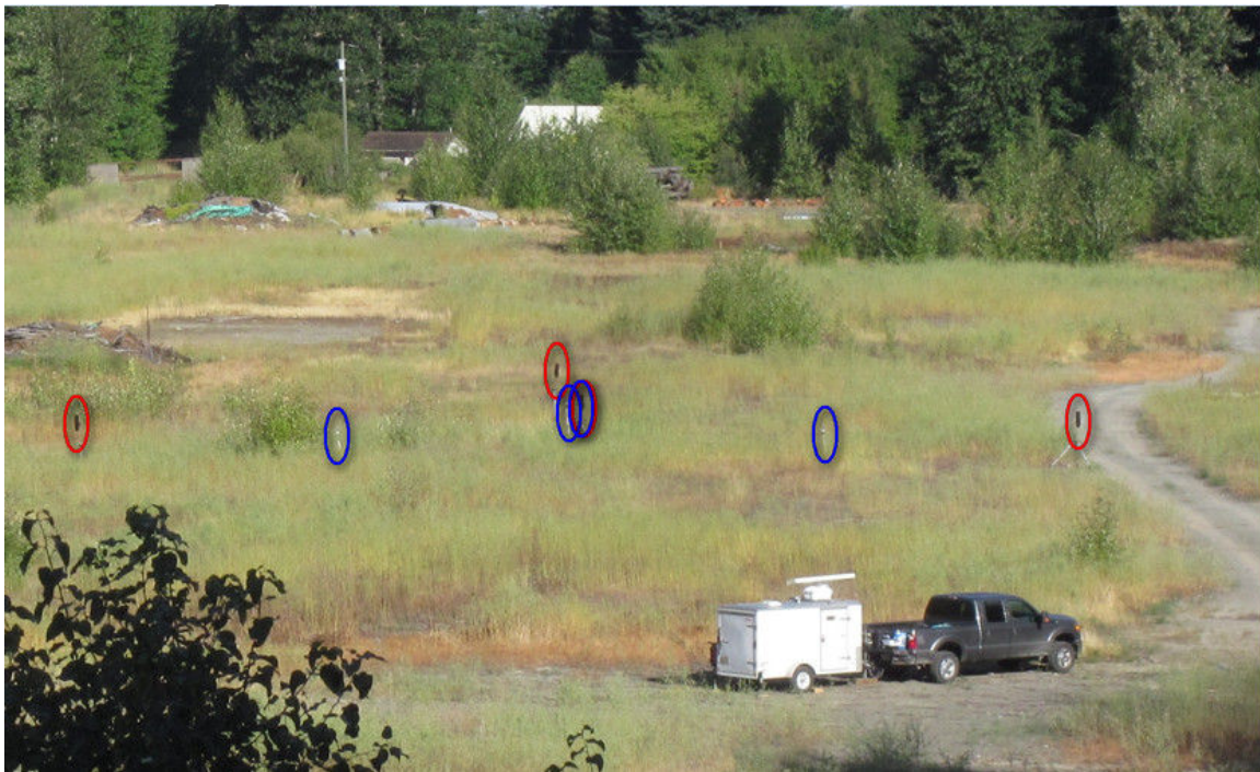
Figure 2.3. Photo showing the setup of the EchoTrack System with the use of both acoustic arrays positioned ~90 m perpendicular to the trailer. The bird microphones are shown by red circles and the EchoTrack omni-directional bat sensors are shown with the blue circles.
