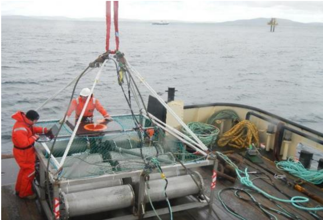
Figure 6: The FLOWBEC monitoring frame being deployed at the EMEC Fall of Warness test site (photo courtesy of Dr Beth Scott)
