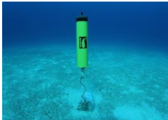
Figure 8: SM2M autonomous marine recorder (photo courtesy of Wildlife Acoustics Inc.)
