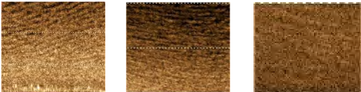
Figure 9: 5m x 5m sections of rippled sand with an altitude of 1.3m and a range of 6m (left) and 10m (middle) and with the sidescan deployed normally and a range of 20m (right).
