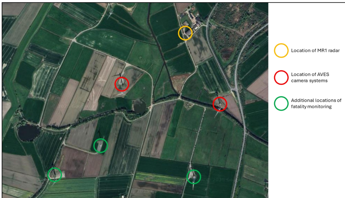
Figure 3-4 Study site with location of radar (yellow), wind turbines equipped with AVEs camera systems, and additional turbine locations used for fatality monitoring.
