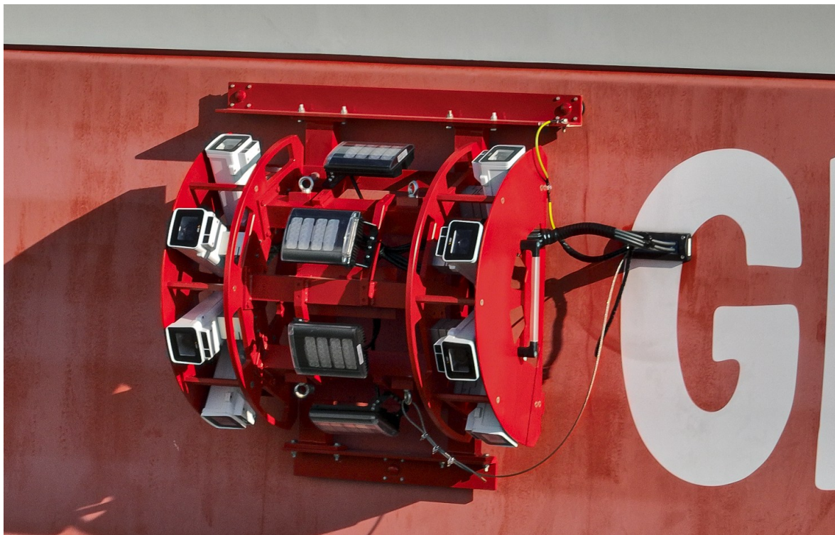
Figure 3-5 The AVES Offshore HPC system, consisting of four stereo-vision camera pairs and infrared light sources to facilitate bird detection at night.
