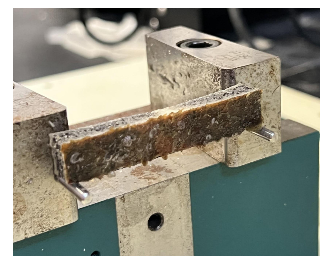
Figure 2. Turtle shell sample on the impact testing device. Samples include all bone layers and keratin; Potential energy for all tests was 2.77 J while hammer speed was ~3.6 m/s.
