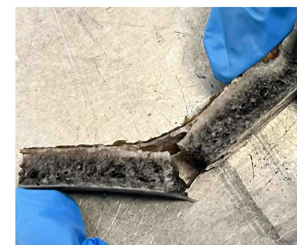
Figure 3. Fractured shell sample after impact testing. Note that the keratin layer remains intact while the bone breaks upon impact. Bone fracture through all layers has been seen in 100% of samples tested to date
