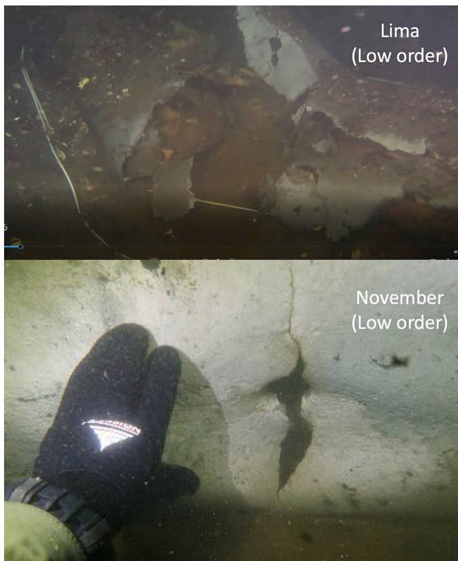
Fig. 19. Post clearance of images of two low-order events LIMA and NOVEMBER showing impact of low-order deflagration on the mine casing.
