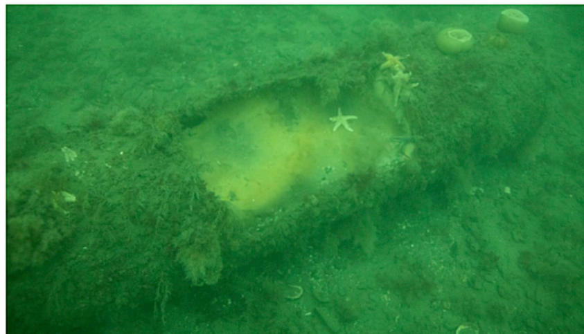
Fig. 1. GOLF – identified as British Mk 1–4 mine (340 kg). Pre-clearance survey shows heavy marine growth and Amatol explosive exposed to the environment..
