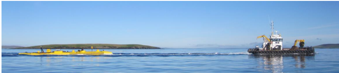
Figure 4.8 Multi-cat workboat towing SR250 turbine
