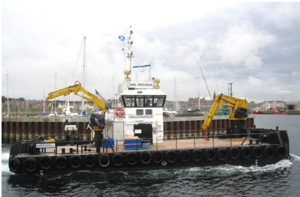
Figure 4.7 Typical multi-cat workboat vessel
