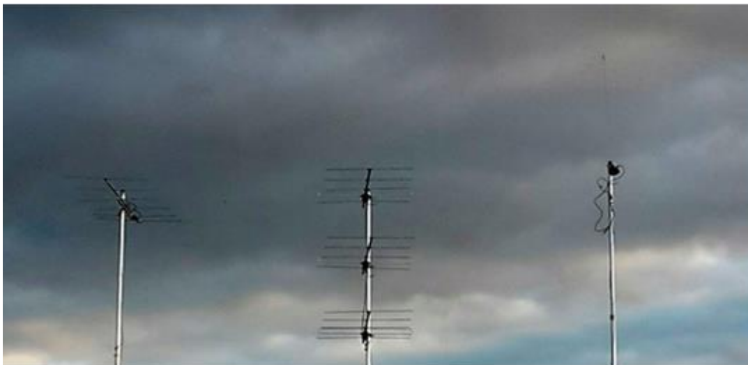
Figure 2.3: 6-element Yagi (left), 5-element Yagi (centre) and the omnidirectional antenna (right). In this experiment the signal of the upper 5-element Yagi was used.
