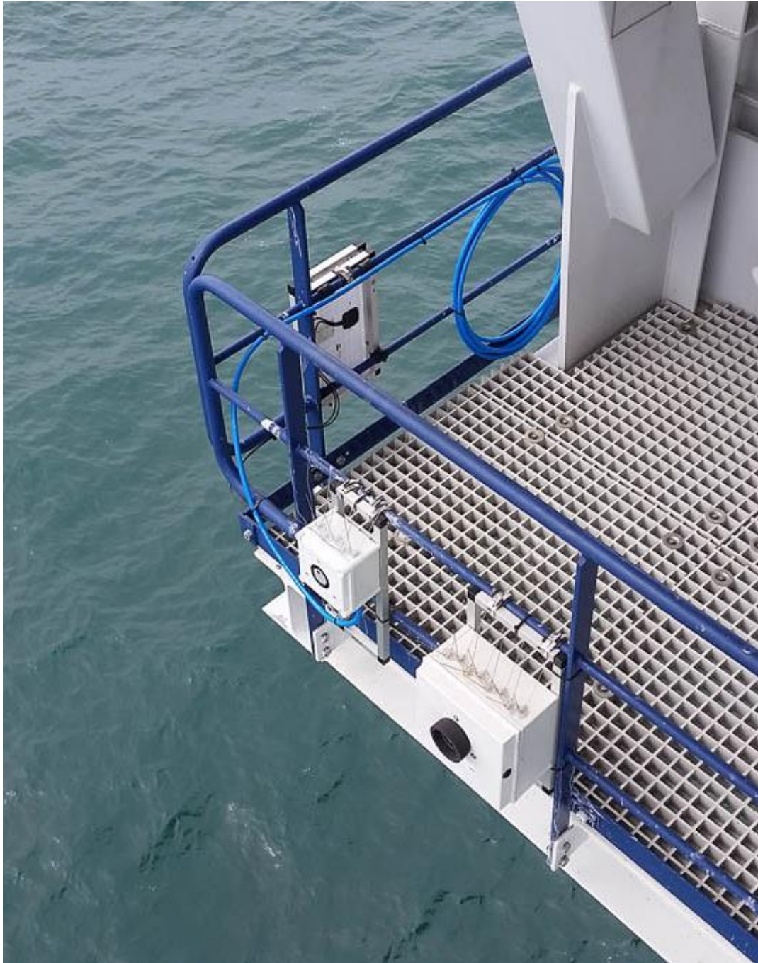
Figure 2.3 Avisoft detector (left) and Batcorder (right)
