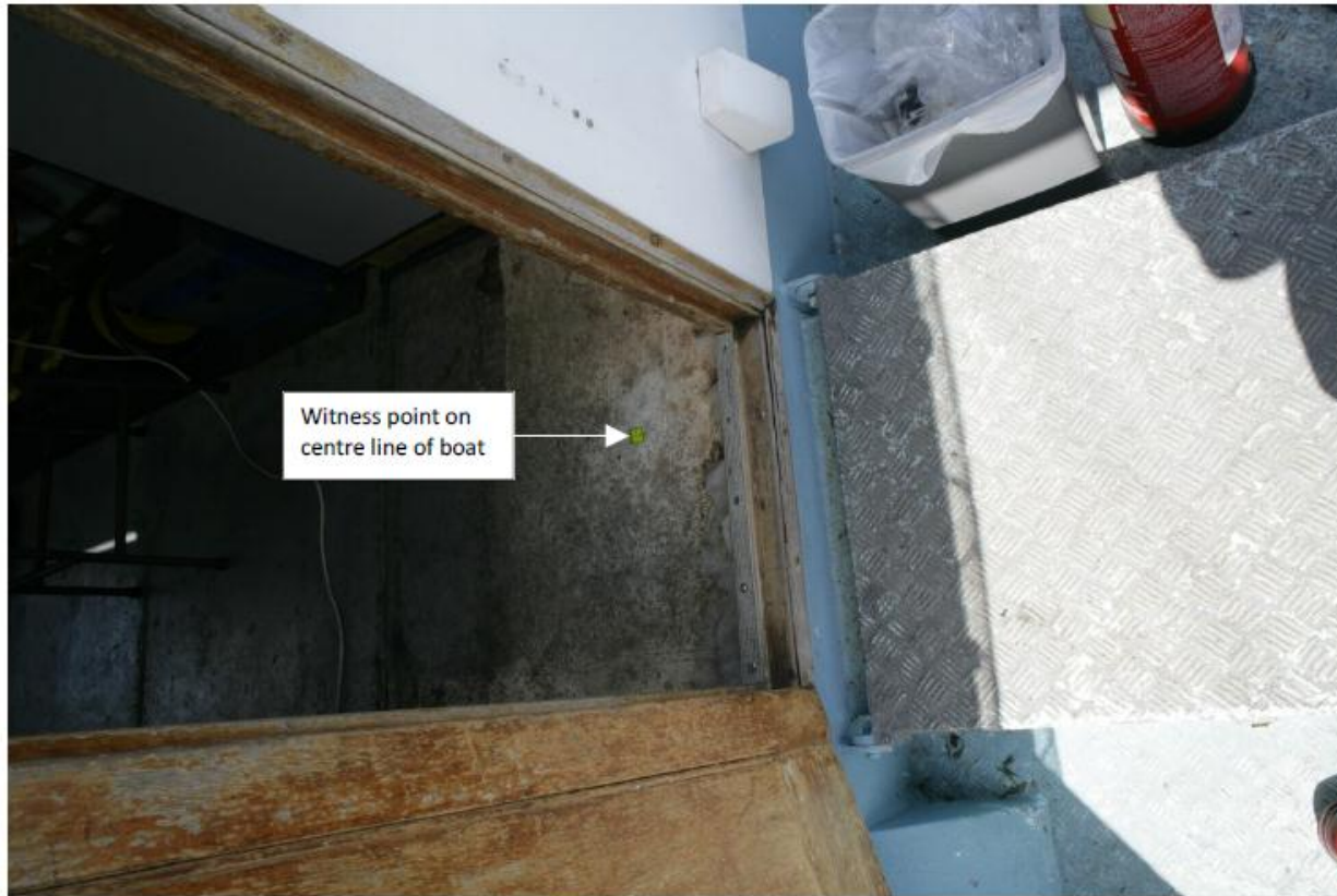
Interior Witness Mark
