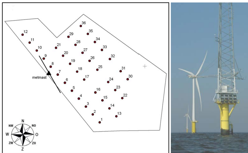
Figure 2.2 Outline of the wind farm with the position of the metmast (triangle) as well as orientation of the vertical radar beam (black line through metmast). Photograph shows the metmast from the south and two wind turbines (Photo: K. Krijgsveld).
