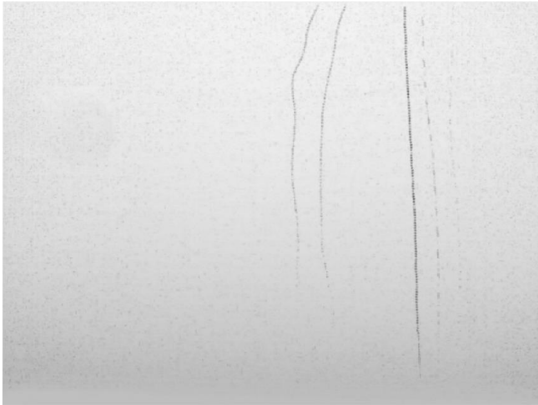
Figure 4 Summary image of a high-confidence collision on March 18 2025, consisting of tracks of multiple objects falling down simultaneously. Because there was no visual corroboration from the upward looking cameras, this was not classified as a confirmed collision. Colours are inverted from the original image for visual clarity.
