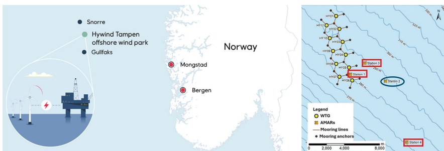
Fig. 1 Location of Hywind Tampen in the North Sea and the producing oil and gas fields “Snorre” and “Gullfaks” that Hywind Tampen powers (left). (©with permission from Equinor ASA). Red dots onshore indicate Norwegian cities. Right: deployment location of JASCO's Autonomous Multichannel Recorders (AMARs) at Hywind Tampen, showing relative positions to wind generator turbines (WTG) and the mooring system. Red rectangle: equipment retrieved after 3 months; blue oval: equipment retrieved after 13 months and not part of this study, but details can be found in Welch et al. 2025
