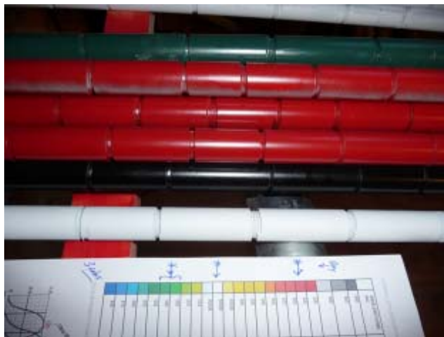
Figure 5. PVC Rope mimics used in the vision experiments with a color spectrum chart to show color frequencies. (Orange “ropes” not shown)
