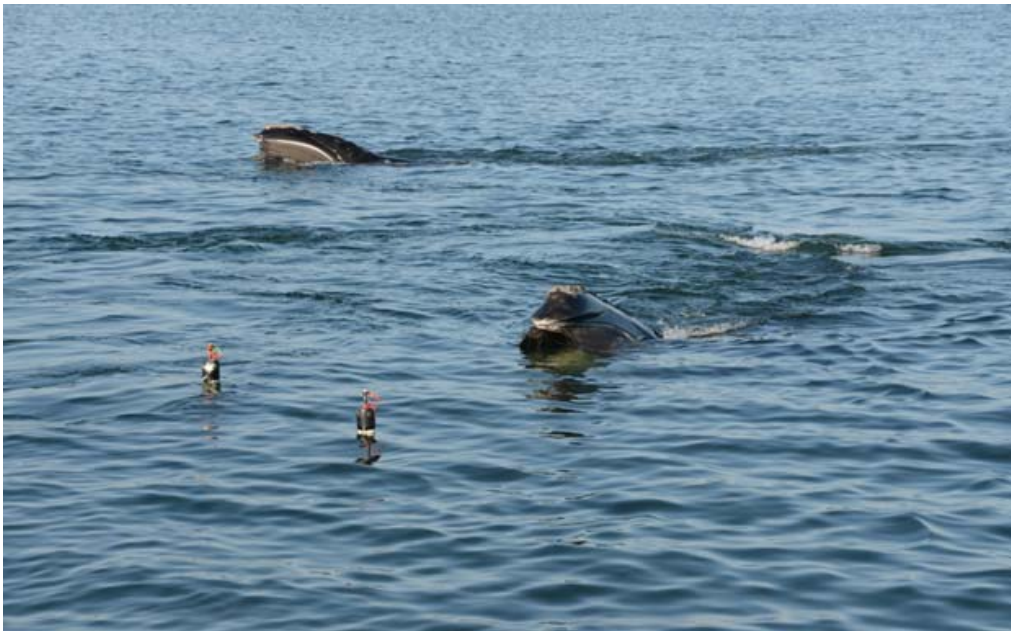
Figure 7. Example of a whale encounter with fake ropes. Whales are skim-feeding from right to left. Lobster bouys are connected to 20 feet of scored and colored 1 inch PVC pipe hanging vertically in the water column. These two buoys/rope-mimics were uncharacteristically close together because of differential drift patterns during a longer deployment.
