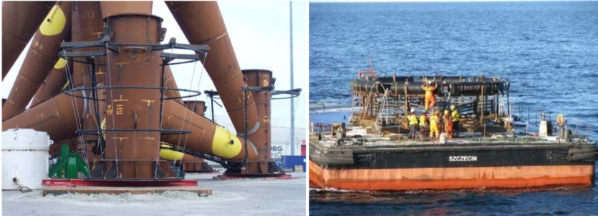
Figure 10: Little bubble curtain, layered ring system. Left: Tripod for the OWF alpha ventus with pre-installed lower unit (source: Hydrotechnik Lübeck GmbH in: GRIEBMANN et al. 2010). Right: Transport of mobile unit to the OWF Baltic II (source: ZERBST & RUSTEMEIER 2011)
