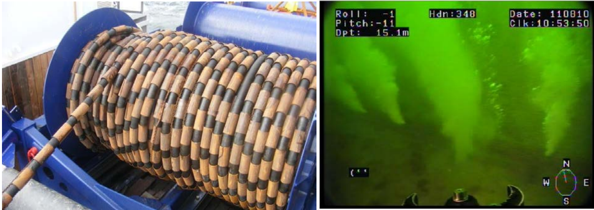
Figure 5: BBC by Hydrotechnik Lübeck as applied at the OWF Borkum West II . Winch with nozzle pipe on pipe-laying vessel (left), and underwater photo during test in the Baltic Sea (right) (source: PEHLKE et al. 2012)
