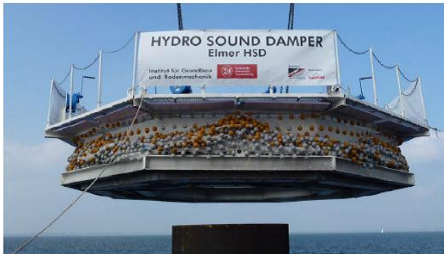
Figure 27: HSD-Platform above the test pile (source: WILKE et al. 2012, photo: Patrice Kunte)
