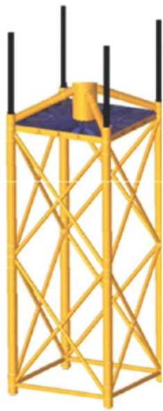
Figure 26: Concept of a quadjack foundation with Pile-in-Pipe Piling for the application with an offshore wind turbine (source: OVERDICK GmbH & Co. KG, Hamburg, modified)
