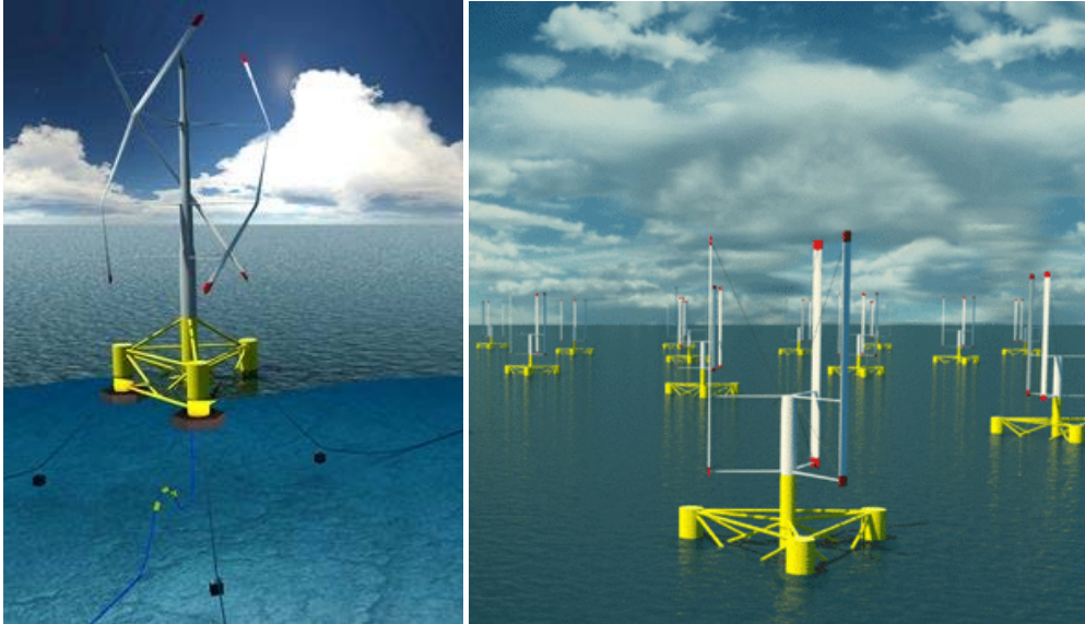
Figure 59: The distinguishing feature of Technip's INFLOW project is the vertical axis wind turbine resulting in a low centre of gravity (source: www.inflow-fp7.eu )
