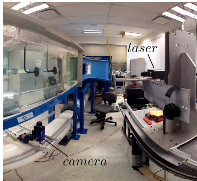
Figure 3-6: Experimental setup. The camera and laser were mounted on rails to facilitate efficient collection of PIV data over the entire test section width and length.
