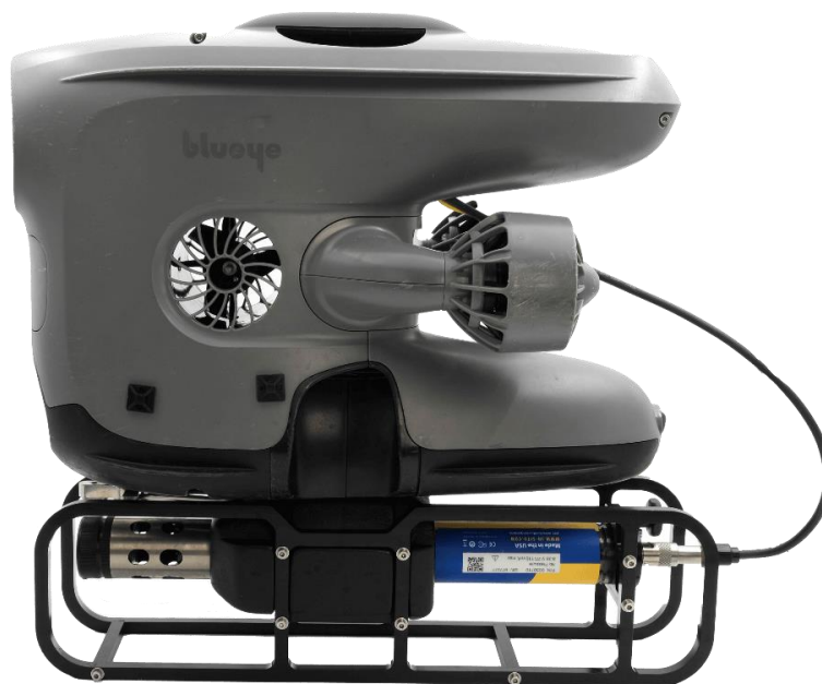
Figure 19. Aqua TROLL 500 in a skid mounted under a Blueye Robotics ROV 19 .
