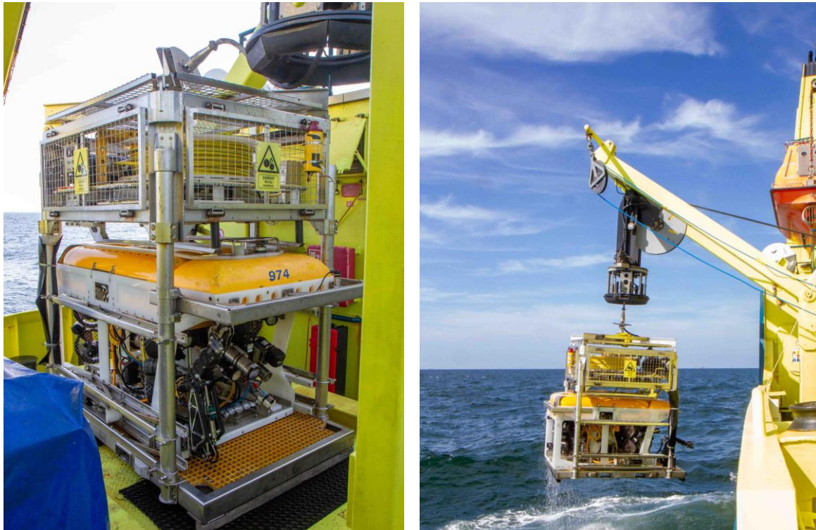
Figure 4. Compact work class ROV (Saab Seaeye Panther ROV equipped with a 4K resolution SUB-C camera) used for video monitoring of the Dutch North Sea, in a LARS system, onboard the RWS ship ARCA, during the MONS Borkum Reef monitoring in August 2024 (photos: Oscar Bos, WMR).
