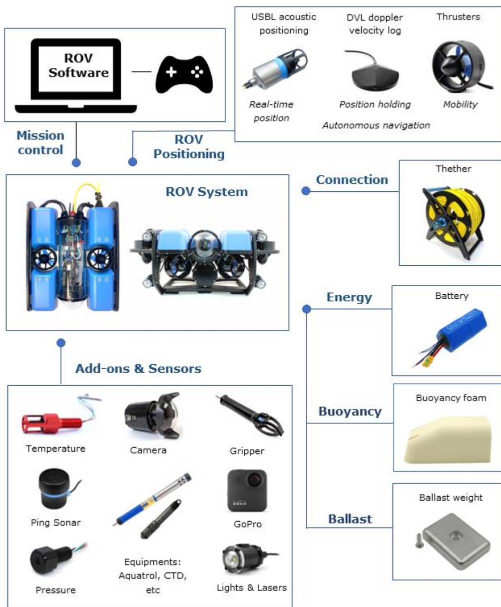
Figure 5. Structure and components of a Handheld ROV: BLUEROV2 7 .
