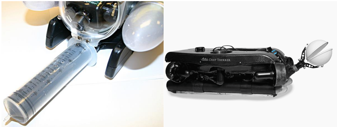
Figure 13. Configuration water samplers on ROVs: VideoRay water sampler 100 mL 12 (left). DeepTrekker water sampler 1L 13 (right).
