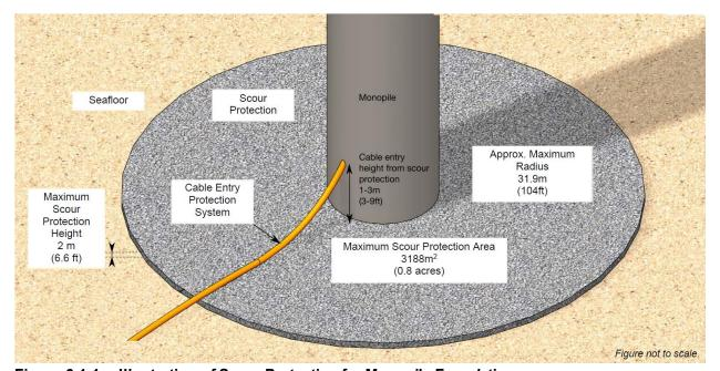
Figure 6.1-1 Illustration of Scour Protection for Monopile Foundation
