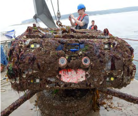
Figure 15 - Example of extreme biofouling from recent AMP deployment with UV lights on sonar transducers
