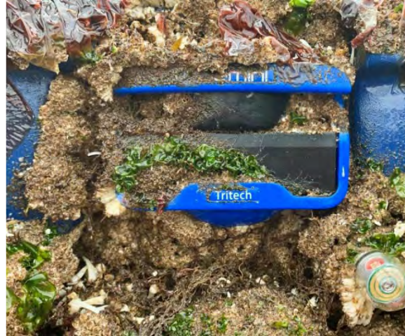
Figure 15 - Example of extreme biofouling from recent AMP deployment with UV lights on sonar transducers
