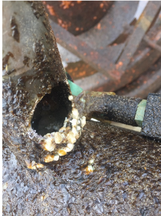
Examples of corrosion on anodized aluminum housing and connectors with dissimilar metals
