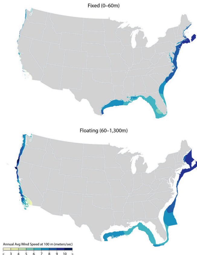
FIGURE 1 | Offshore wind speeds in the US waters, split by technology type.
