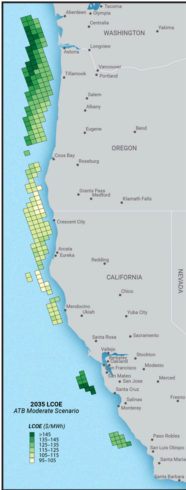
FIGURE 2 | Offshore wind levelized cost of energy (LCOE) distribution for the West Coast. This represents 2035 costs from the moderate cost trajectory from NLR's Annual Technology Baseline (ATB) 2024 [24]. Note: The map shows only sites considered under the reference access case from [43].
