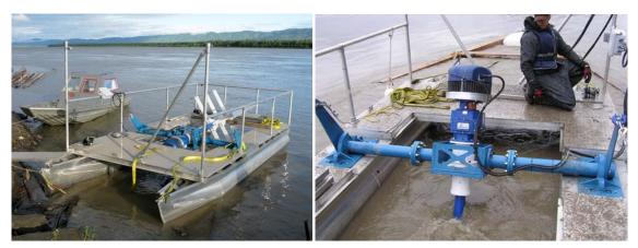
Figure 6. New Energy EnCurrent Turbine (on left) and deployed in the Yukon River (pictures courtesy of New Energy Corporation and Tom Ravens)
