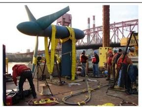
Figure 10. Propeller blade horizontal axis turbine (photo courtesy of Verdent Power)
