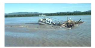
Figure 14. Debris pile on a 5 kW turbine barge at Ruby, Alaska
