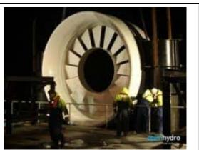
Figure 9. Open-Centre Turbine fan blade (photo courtesy of OpenHydro)
