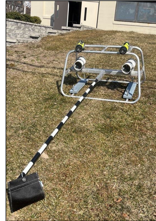
Figure 2-2. Primary field sampling equipment; (A) CastAway CTD; (B) Kemmerer sampling bottle for eDNA collection; (C) stereo BRUV system. Stereo BRUV systems include a subsea lighting setup, two GoPro HERO11 video cameras with SeaGIS camera housings, weights, a bait arm, and a bait bag.
