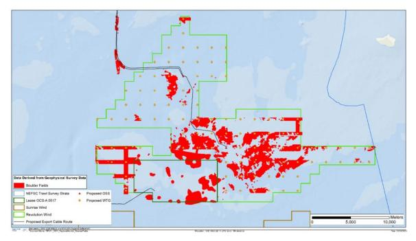
Figure 2. Locations of boulder fields within the RWF and SFW lease sites, and along the RWEC corridor, that were mapped during high-resolution geophysical surveys conducted by Ørsted.
