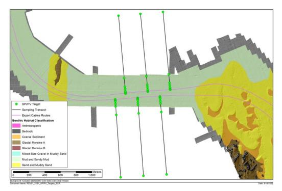
Figure 22. Conceptual diagram of the proposed soft bottom benthic survey sampling design within one habitat stratum along the RWEC with green dots indicating SPI/PV stations situated along transects perpendicular to the RWEC, and independent triplicate transects sampled in both directions.
