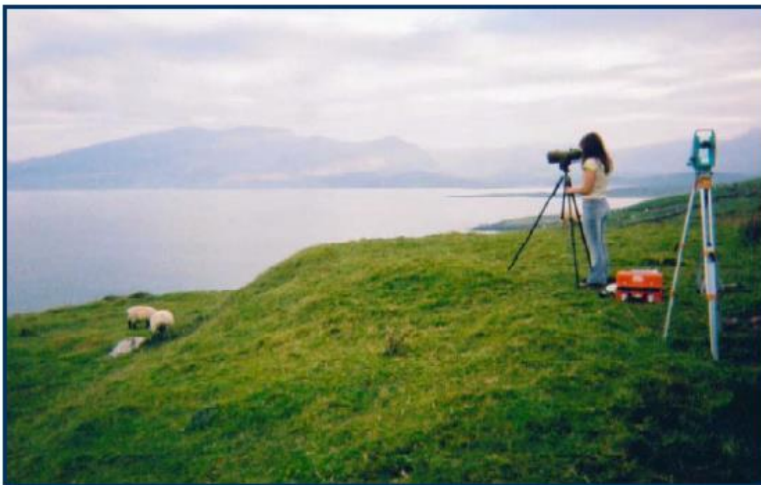
Figure 1. Shore based surveys for marine mammals showing an observer scanning the sea surface using a 30x telescope. The theodolite is shown set up ready for use in the foreground. (from Ingram et al. , 2005).
