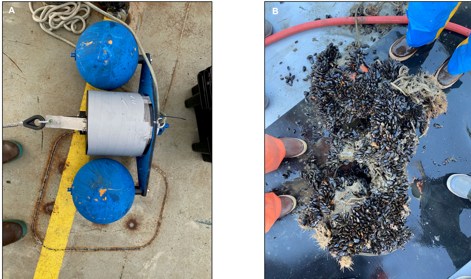
Figure 3-3. Comparison of an Innovasea VR2AR acoustic receiver with a recoverable acoustic release mooring system (A) before and (B) after deployment in terms of biofouling. All receivers and mooring systems are treated with an antifouling ablative paint to inhibit growth prior to release.
