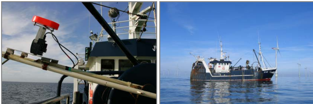
Photo 1-2. The 4x10, 120KHz transducer and pan & tilt unit was mounted by a specially designed device on the port side of the vessel "MS Juli-Ane".
