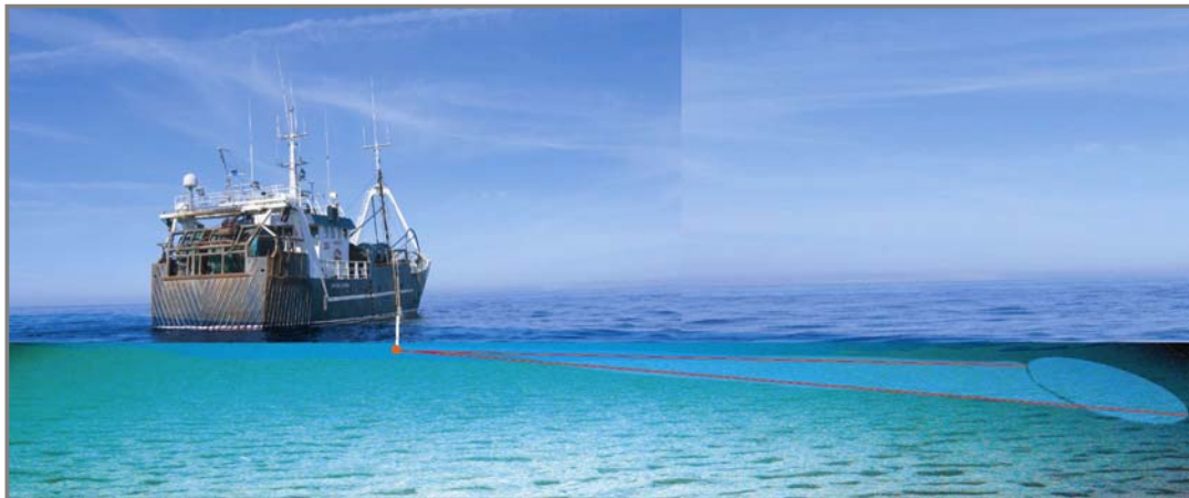
Figure 3.1. Illustration showing the spatial distribution of horizontal hydroacoustic beam
