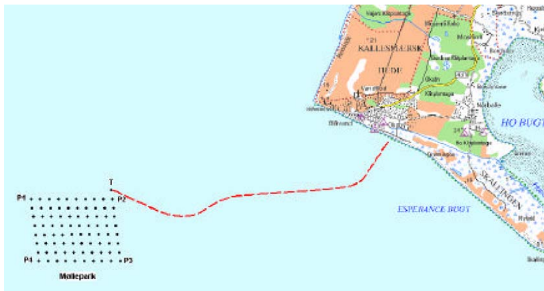
Figure 2.1. The offshore wind farm at Horns Rev and the cable trace to land at Hvidbjerg Strand. T marks the transformer platform.
