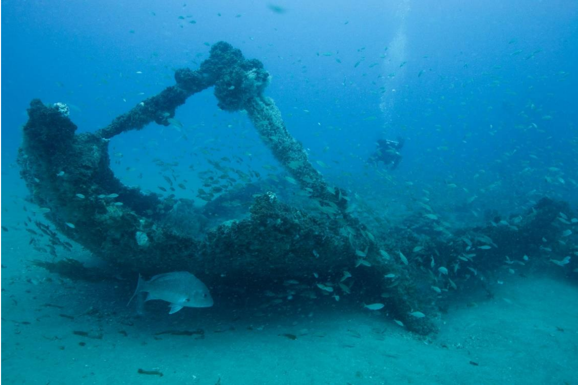
Figure 42: Stern section of City of Houston with potential rudder post remains.
