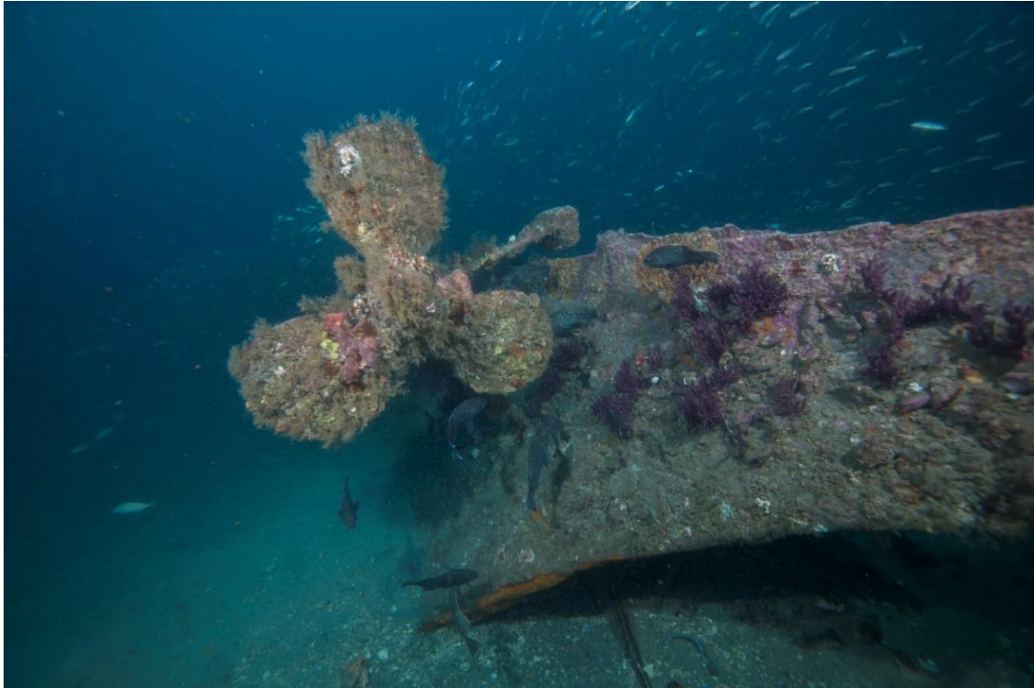
Figure 17: Port propeller and shaft of 6537K_1.
