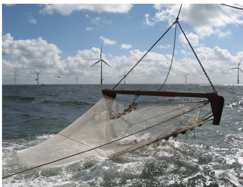
Figure 3.1: One of the 6 m beam trawls used for sampling the demersal fish community. Attached is the 20 mm net. In the middle of the net the CTD device is visible. (photo: R. ter Hofstede).
