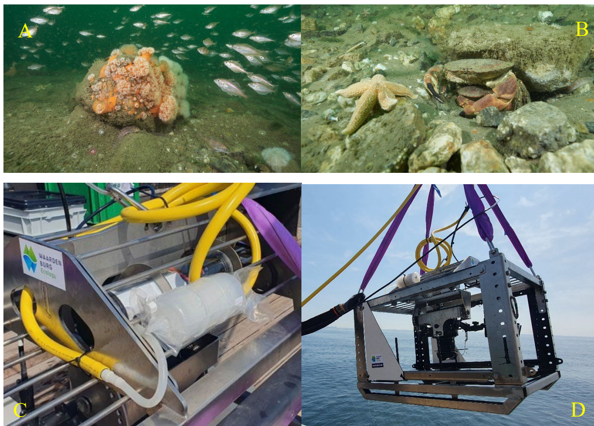
Figure 3 - Overview of cable crossings showing (A) an armour layer rock (D90 400mm) covered with marine growth and (B) different types of sprinkle layer (D90 80mm) with a Edible crab ( Cancer pagurus ) and a common starfish ( Asterias rubens ), source: DPM. Monitoring techniques used on the cable crossings showing (C) the dropcam frame with the camera mounted in the center and (D) the pump used to collect water for eDNA analysis.
