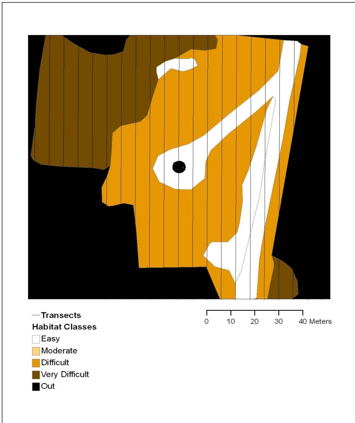
Figure 2. Example carcass search plot at a wind turbine depicting the maximum plot size of 126 m east-west and 120 m north-south, 6 m wide transect lines (searched 3 m on each side), unsearchable area (black), and area encompassed by easy (white), moderate (light tan), difficult (dark tan), and very difficult (brown) visibility habitat.
